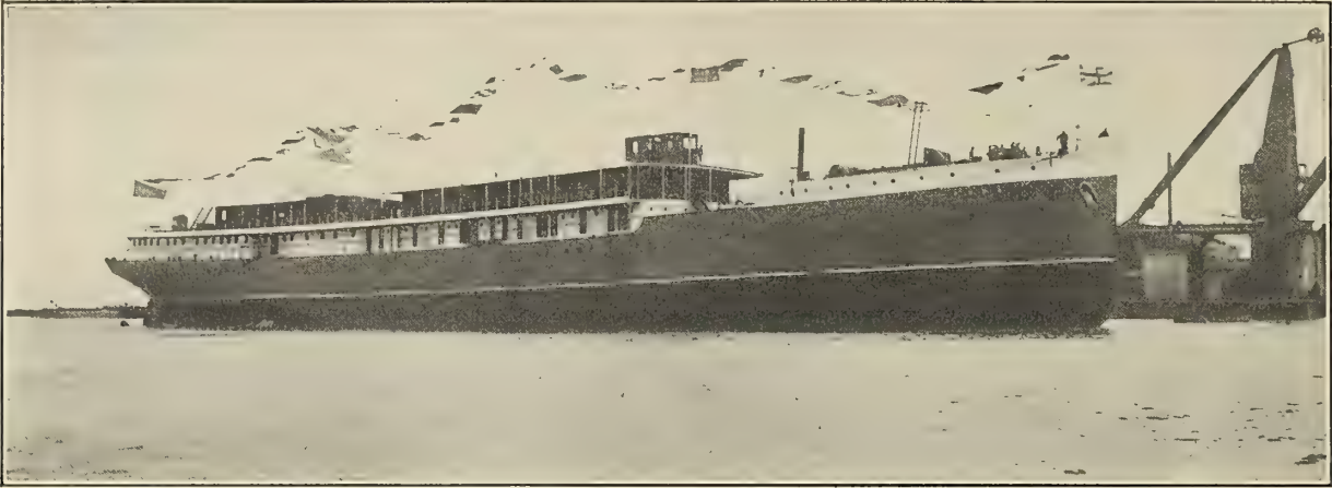
THE SHIP AFLOAT AFTER LAUNCHING, AND READY FOR RECEIVING MACHINERY AND FITTINGS.
